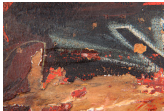
Fig.10 - Microscopic images pointing the top blue layer on the cloth and the bottom red layer underneath
