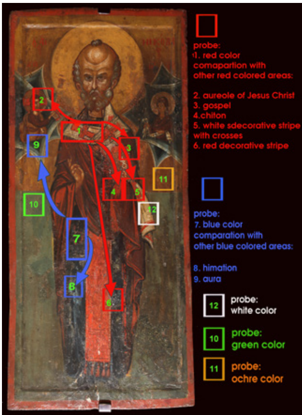
Fig. 9 – Measurement points analyzed with the e X-ray fluorescence analyses
